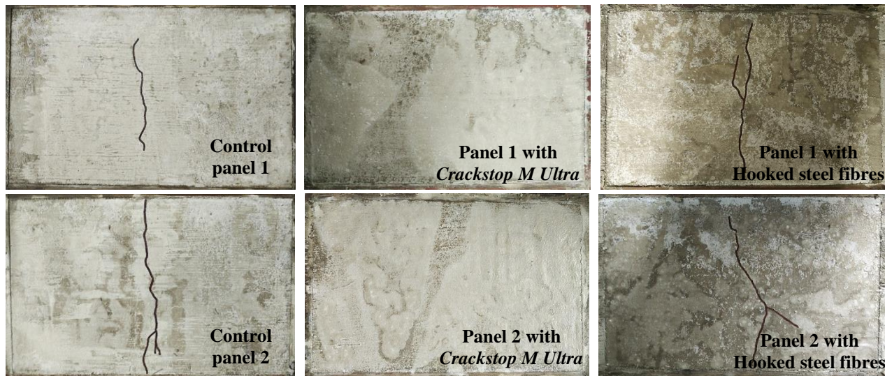
Fig. 5. Final crack patterns
