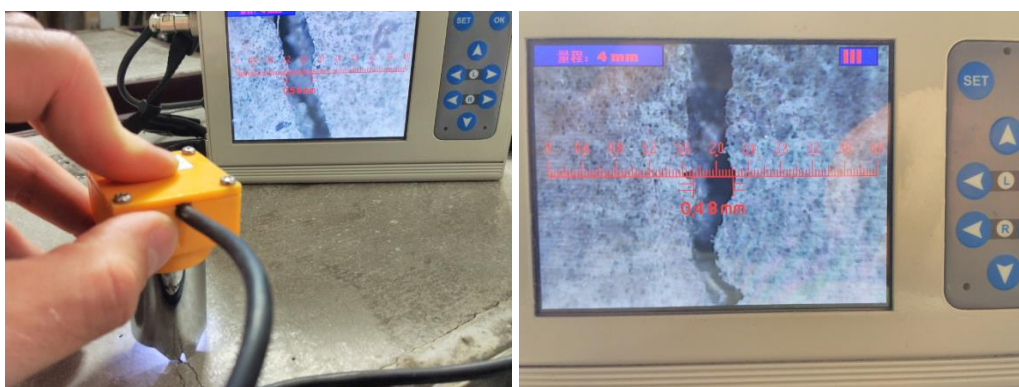
Fig. 4. Crack width measurement
